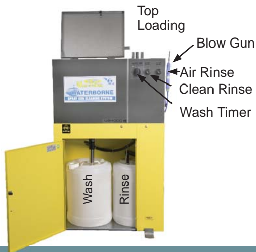
DIAPHRAGM PUMP POWERS the UA400W
